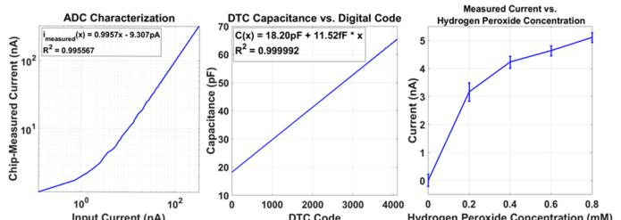
Fig.4 In-vitro hydrogen peroxide potentiostat measurements and characterization
