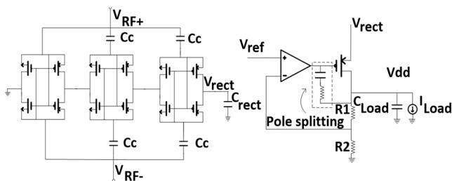
Fig.3 Circuit topologies of rectifier and LDO
