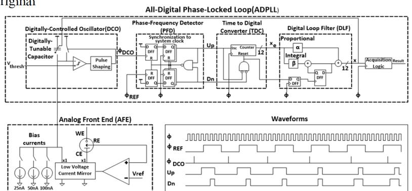
Fig.2 Architecture of the ADPLL based potentiostat
