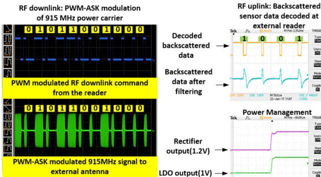
Fig.5 Power management and data telemetry measurements
