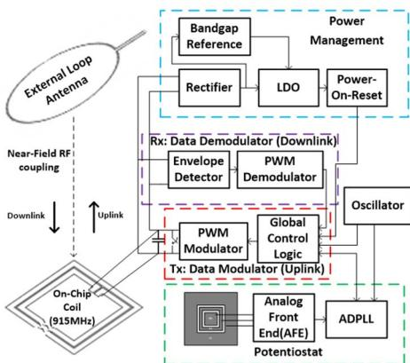
Fig.1 Block diagram of the implantable potentiostat system
